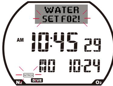
When the FO2 is not set (i.e. default value is used), an alarm will sound when dive mode starts and display blinks until FO2 is set.
