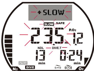
Whenever the ascent rate is too fast for a particular depth, COMPASS + will give out an audible alarm and its display will flash. If the surfacing speed is not reduced to within an acceptable level, the unit will continue sounding the alarm and will only stop when the depth is shallower than 1.2m (4 feet). This information is recorded in the dive log when the second warning appears within 6 seconds of the first warning. This applies to both DIVE and GAGE mode.
