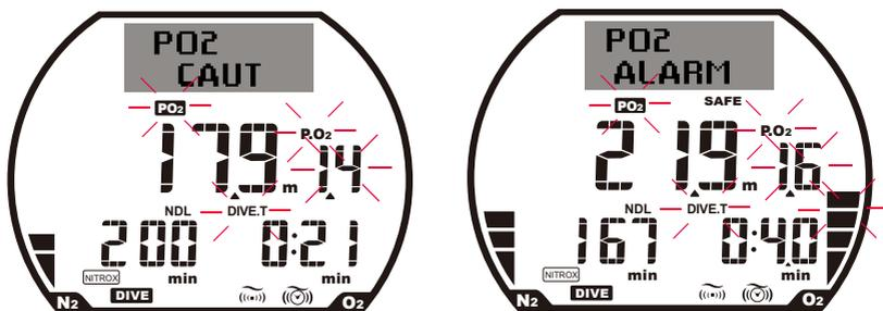
When the partial pressure of oxygen warning comes on, it can mean the PO2 at the current depth is greater than the maximum value set before a dive or PO2 is simply over 1.6.
