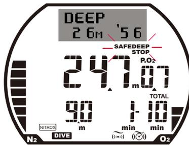
This dive computer has a DEEP STOP function. It is shown only under the decompression mode and may require the diver to stay deeper than 21 meter. One-minute stop(s) will be prescribed (much like a safety-stop) but in a deeper area.
