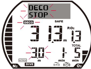
When the NDL is exceeded, COMPASS + automatically changes the mode to decompression dive mode. Warning will be generated and this information is recorded in the dive log.
