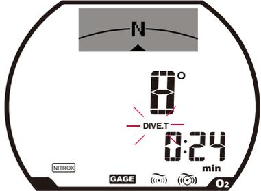
Use the digital azimuth like a conventional compass.
