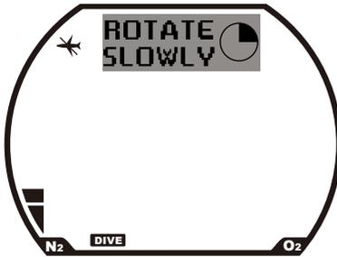
To realign the compass to earth's axis, press the C button for 2 seconds, hold COMPASS + parallel to the ground then rotate the unit very slowly clockwise until a full circle is indicated by the dot-matrix display. Press C for 2 further seconds to exit the function.
