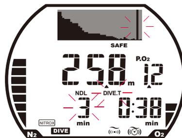
When the ND.L time is counted down to within 3 minutes, a warning is generated. This information is not recorded in the dive log.
