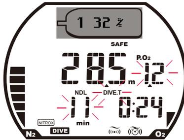
The computer can store up to 3 different Nitrox settings and can be switched from 1 mix to another mid dive, providing that the PO<sub>2</sub> for the gas is under 1.6 at the depth when the switch is made and the oxygen % has been set before a dive began.
