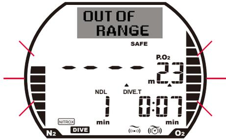
E.g. Water depth exceeds measurement range (deeper than 100m / 328ft)
