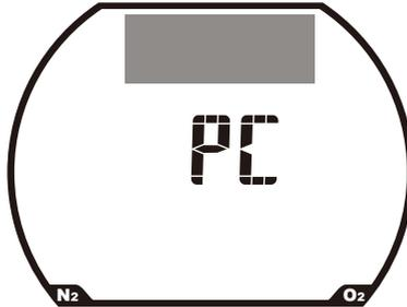
[ Connection between the downloader and COMPASS+ has been established ]
