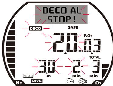
When the depth is shallower than the recommended decompression stop depth, audio and visual warnings will be given once every minute. If the depth is deeper than the prescribed depth, the screen will display normally. This information will be recorded in the dive log.
