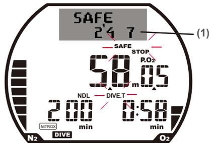
This shows the recommended safety stop time. If the user descends below 9.9m, upon returning to a depth of 6m, this value appears instead of NDL. The safety stop timer starts counting down from 3 minutes to 0:00. Then safety stop timer icon and NDL reappears.
